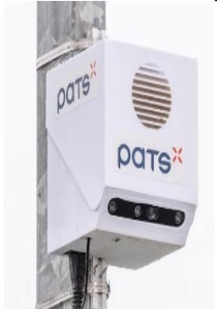
PATS-C camera to detect moths
