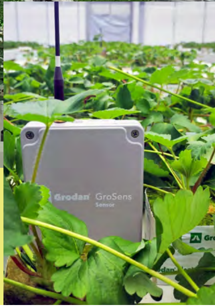
Picture 2. GroSens sensor in a block on an ebb-flood bench during propagation of strawberry.
